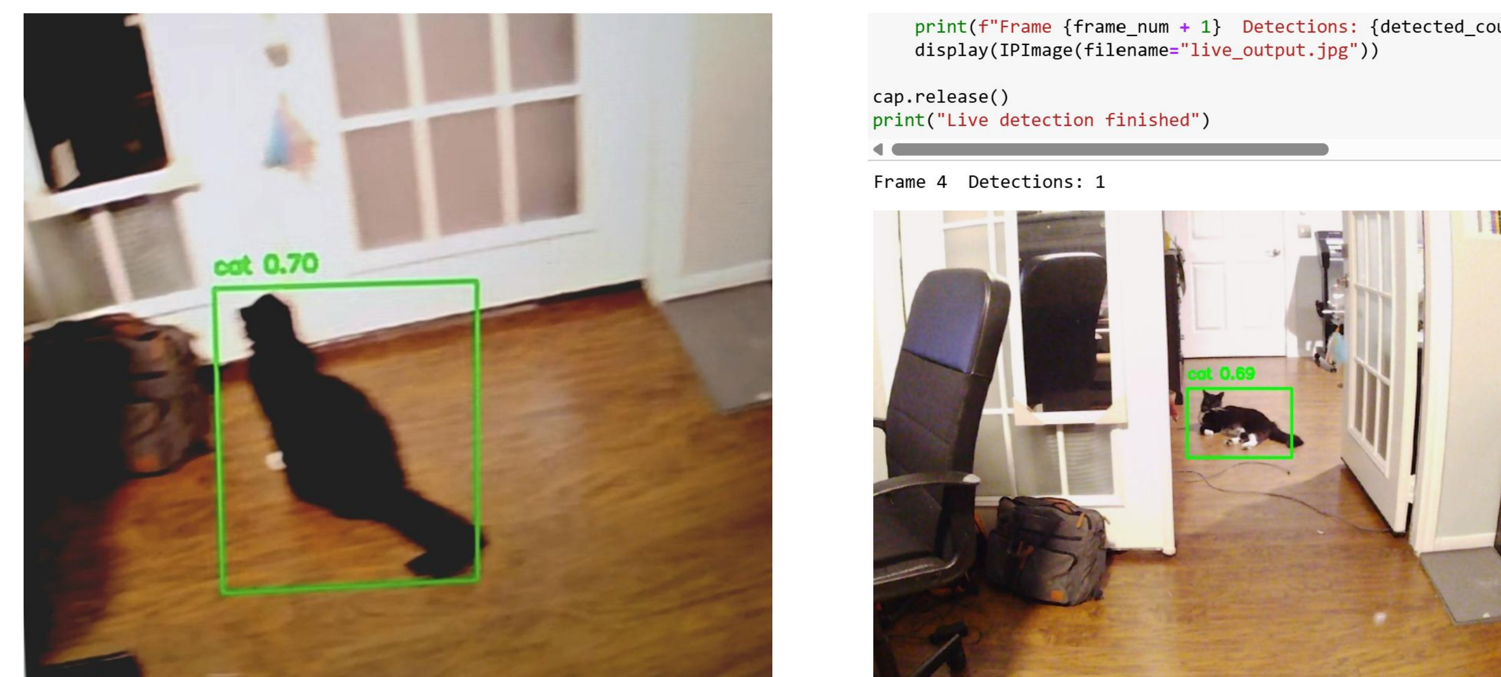
Object Detection Results Using Tiny YOLO
